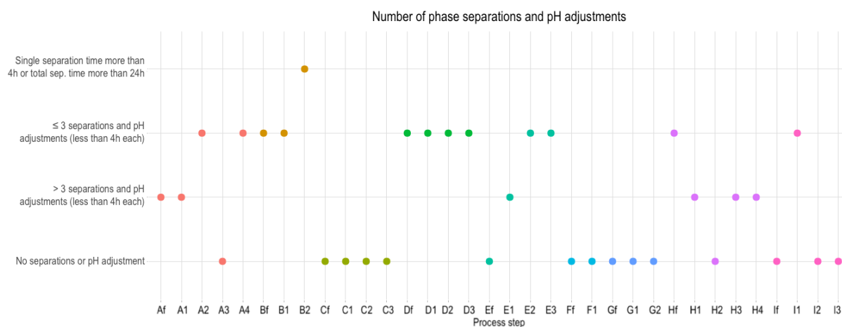
Figure 3.20: Data plot with answers for number of phase separations and pH adjustments for each process step evaluated with the knowledge-based assessment tool, provided by the user interface. Each colour designates one project.
